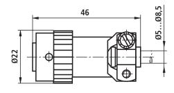
Plug-in connector, separate order stating Material no. **R901043330**
