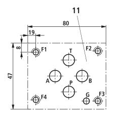
**Subplates** according to data sheet RE 45052 (separate order)
